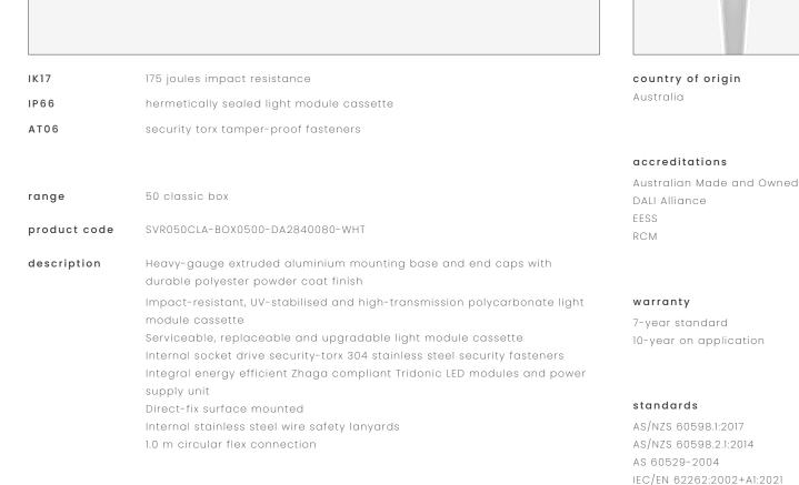
applications extremely robust surface mounted luminaire that enhances safety and security in the most challenging environments. a durable construction ensures dependable operation and superior performance under harsh operating conditions; ideal for applications such as transportation, custodial, public areas, and secure healthcare
