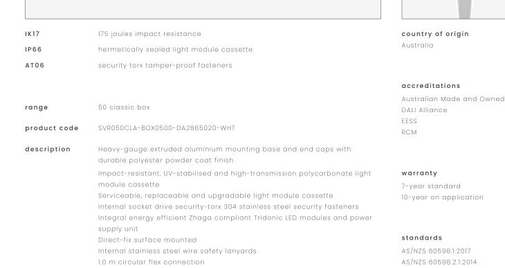
applications extremely robust surface mounted luminaire that enhances safety and security in the most challenging environments. a durable construction ensures dependable operation and superior performance under harsh operating conditions; ideal for applications such as transportation, custodial, public areas, and secure healthcare
