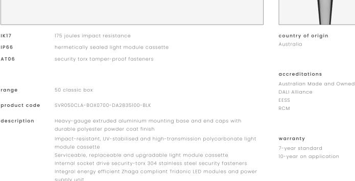
supply unit Direct-fix surface mounted Internal stainless steel wire safety lanyards 1.0 m circular flex connection
