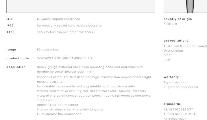
applications extremely robust surface mounted luminaire that enhances safety and security in the most challenging environments. a durable construction ensures dependable operation and superior performance under harsh operating conditions; ideal for applications such as transportation, custodial, public areas, and secure healthcare
