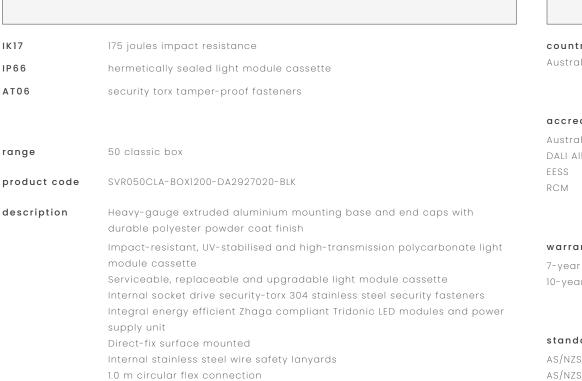
applications extremely robust surface mounted luminaire that enhances safety and security in the most challenging environments. a durable construction ensures dependable operation and superior performance under harsh operating conditions; ideal for applications such as transportation, custodial, public areas, and secure healthcare
