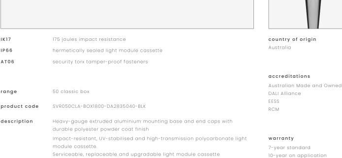
Serviceable, replaceable and upgradable light module cassette Internal socket drive security-torx 304 stainless steel security fasteners Integral energy efficient Zhaga compliant Tridonic LED modules and power supply unit Direct-fix surface mounted Internal stainless steel wire safety lanyards
