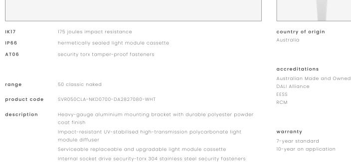
Integral energy efficient Zhaga compliant Tridonic LED modules and power supply unit Direct-fix surface mounted
