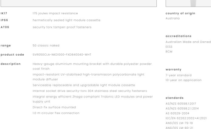
applications extremely robust surface mount luminaire that enhances safety and security in the most challenging environments. a durable construction ensures dependable operation and superior performance under harsh operating conditions; ideal for applications such as transportation, custodial, public areas, and secure healthcare
