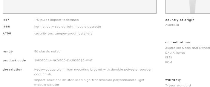
Serviceable replaceable and upgradable light module cassette Internal socket drive security-torx 304 stainless steel security fasteners Integral energy efficient Zhaga compliant Tridonic LED modules and power supply unit Direct-fix surface mounted 1.0 m circular flex connection
