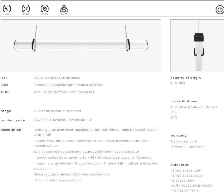
applications extremely robust suspended mount luminaire that enhances safety and security in the most challenging environments. a durable construction ensures dependable operation and superior performance under harsh operating conditions; ideal for applications such as transportation, custodial, public areas, and secure healthcare
