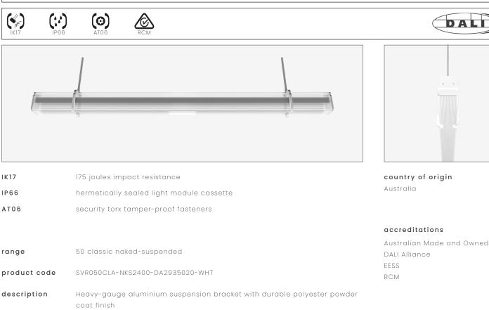
Impact-resistant UV-stabilised high-transmission polycarbonate light module diffuser
