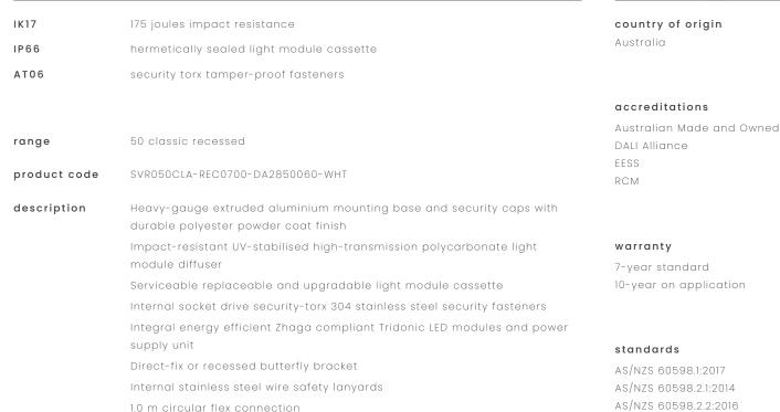
applications extremely robust recessed mount luminaire that enhances safety and security in the most challenging environments. a durable construction ensures dependable operation and superior performance under harsh operating conditions; ideal for applications such as transportation, custodial, public areas, and secure healthcare
