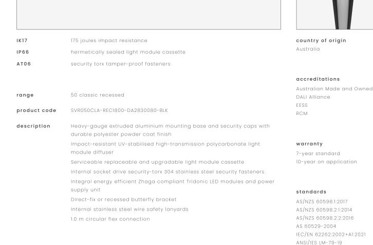
applications extremely robust recessed mount luminaire that enhances safety and security in the most challenging environments. a durable construction ensures dependable operation and superior performance under harsh operating conditions; ideal for applications such as transportation, custodial, public areas, and secure healthcare
