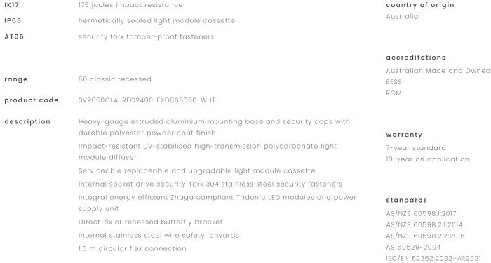
applications extremely robust recessed mount luminaire that enhances safety and security in the most challenging environments. a durable construction ensures dependable operation and superior performance under harsh operating conditions; ideal for applications such as transportation, custodial, public areas, and secure healthcare
