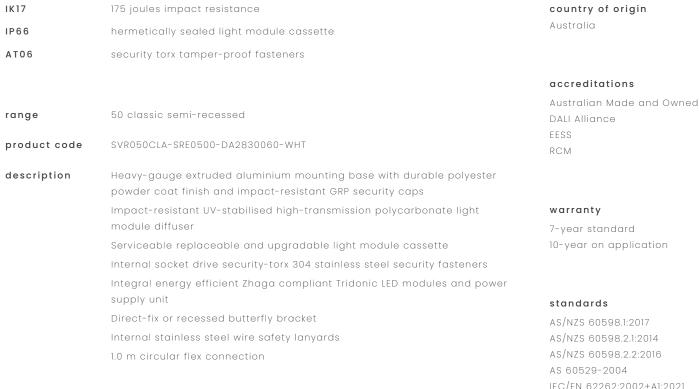
applications extremely robust semi-recessed mount luminaire that enhances safety and security in the most challenging environments. a durable construction ensures dependable operation and superior performance under harsh operating conditions; ideal for applications such as transportation, custodial, public areas, and secure healthcare
