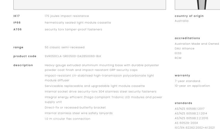
applications extremely robust semi-recessed mount luminaire that enhances safety and security in the most challenging environments. a durable construction ensures dependable operation and superior performance under harsh operating conditions; ideal for applications such as transportation, custodial, public areas, and secure healthcare
