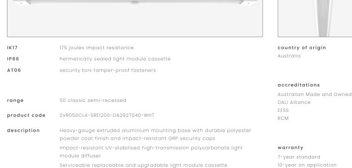
Internal socket drive security-torx 304 stainless steel security fasteners Integral energy efficient Zhaga compliant Tridonic LED modules and power supply unit Direct-fix or recessed butterfly bracket Internal stainless steel wire safety lanyards
