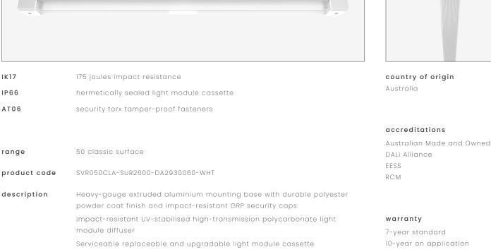
Internal socket drive security-torx 304 stainless steel security fasteners Integral energy efficient Zhaga compliant Tridonic LED modules and power supply unit Direct-fix surface mounted
