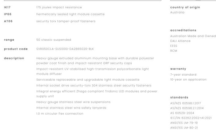
applications extremely robust suspended mount luminaire that enhances safety and security in the most challenging environments. a durable construction ensures dependable operation and superior performance under harsh operating conditions; ideal for applications such as transportation, custodial, public areas, and secure healthcare
