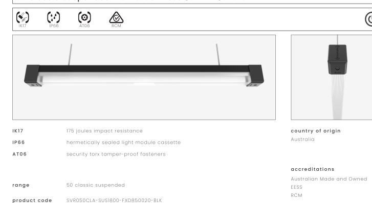
description Heavy-gauge extruded aluminium mounting base with durable polyester powder coat finish and impact-resistant GRP security caps Impact-resistant UV-stabilised high-transmission polycarbonate light module diffuser Serviceable replaceable and upgradable light module cassette Internal socket drive security-torx 304 stainless steel security fasteners Integral energy efficient Zhaga compliant Tridonic LED modules and power supply unit
