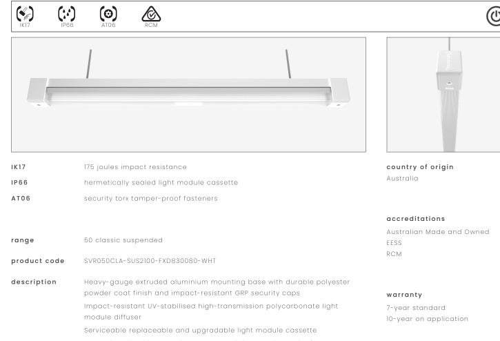
Internal socket drive security-torx 304 stainless steel security fasteners Integral energy efficient Zhaga compliant Tridonic LED modules and power supply unit
