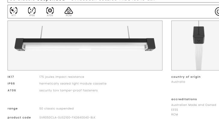
description Heavy-gauge extruded aluminium mounting base with durable polyester powder coat finish and impact-resistant GRP security caps Impact-resistant UV-stabilised high-transmission polycarbonate light module diffuser Serviceable replaceable and upgradable light module cassette Internal socket drive security-torx 304 stainless steel security fasteners Integral energy efficient Zhaga compliant Tridonic LED modules and power supply unit Heavy-gauge stainless steel wire suspensions
