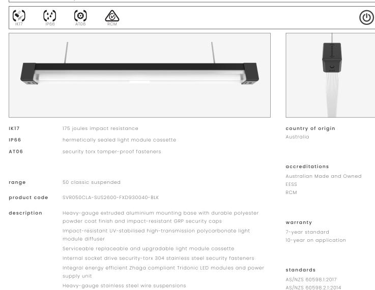
Heavy-gauge stainless steel wire suspensions Internal stainless steel wire safety lanyards 1.0 m circular flex connection
