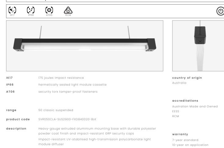
Serviceable replaceable and upgradable light module cassette Internal socket drive security-torx 304 stainless steel security fasteners Integral energy efficient Zhaga compliant Tridonic LED modules and power supply unit Heavy-gauge stainless steel wire suspensions
