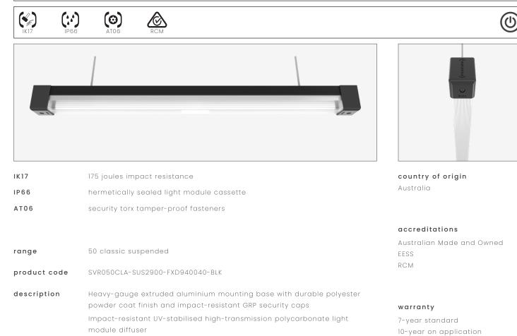
Serviceable replaceable and upgradable light module cassette Internal socket drive security-torx 304 stainless steel security fasteners Integral energy efficient Zhaga compliant Tridonic LED modules and power supply unit Heavy-gauge stainless steel wire suspensions
