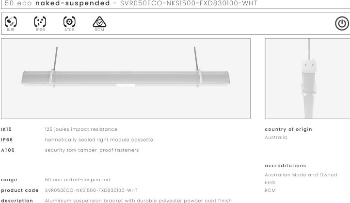
Aluminium suspension bracket with durable polyester powder coat finish Impact-resistant UV-stabilised high-transmission polycarbonate light module diffuser Serviceable replaceable and upgradable light module cassette Internal socket drive security-torx 304 stainless steel security fasteners Integral energy efficient Zhaga compliant Tridonic LED modules and power supply unit Heavy-gauge stainless steel wire suspensions 1.0 m circular flex connection
