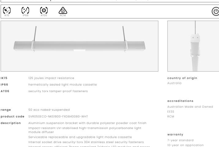
Integral energy efficient Zhaga compliant Tridonic LED modules and power supply unit Heavy-gauge stainless steel wire suspensions 1.0 m circular flex connection
