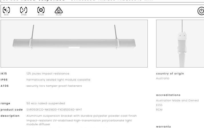
Serviceable replaceable and upgradable light module cassette Internal socket drive security-torx 304 stainless steel security fasteners Integral energy efficient Zhaga compliant Tridonic LED modules and power supply unit Heavy-gauge stainless steel wire suspensions 1.0 m circular flex connection
