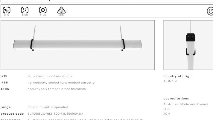
description Aluminium suspension bracket with durable polyester powder coat finish Impact-resistant UV-stabilised high-transmission polycarbonate light module diffuser Serviceable replaceable and upgradable light module cassette Internal socket drive security-torx 304 stainless steel security fasteners Integral energy efficient Zhaga compliant Tridonic LED modules and power supply unit Heavy-gauge stainless steel wire suspensions 1.0 m circular flex connection
