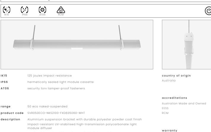
module diffuser Serviceable replaceable and upgradable light module cassette Internal socket drive security-torx 304 stainless steel security fasteners Integral energy efficient Zhaga compliant Tridonic LED modules and power supply unit Heavy-gauge stainless steel wire suspensions 1.0 m circular flex connection
