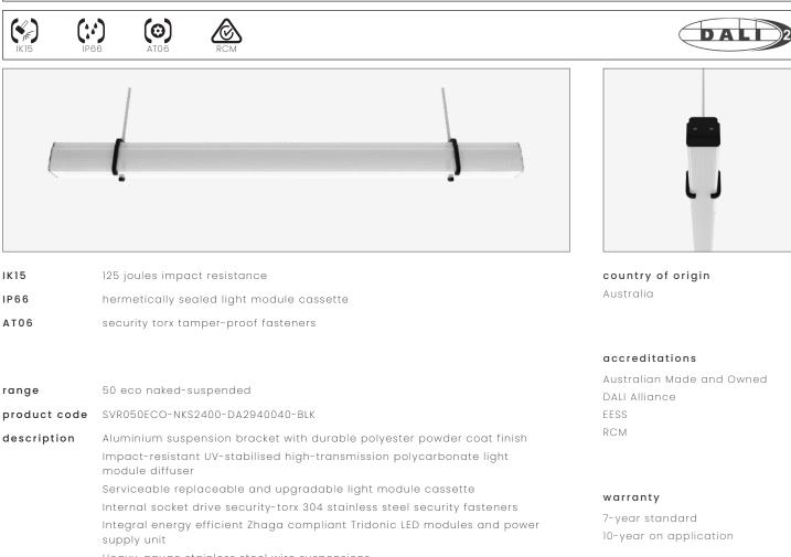
Heavy-gauge stainless steel wire suspensions 1.0 m circular flex connection
