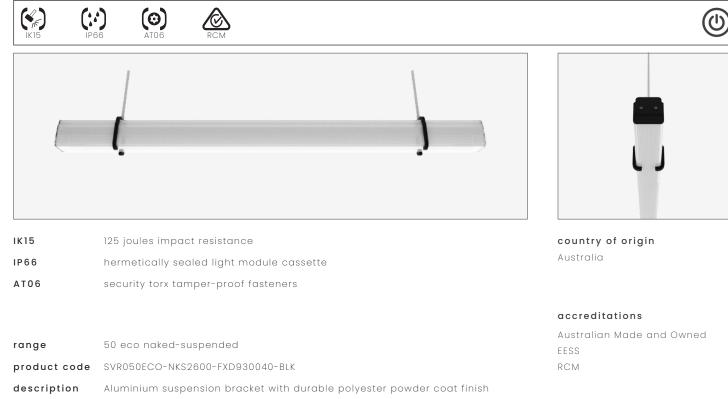
Impact-resistant UV-stabilised high-transmission polycarbonate light module diffuser Serviceable replaceable and upgradable light module cassette Internal socket drive security-torx 304 stainless steel security fasteners Integral energy efficient Zhaga compliant Tridonic LED modules and power supply unit Heavy-gauge stainless steel wire suspensions 1.0 m circular flex connection
