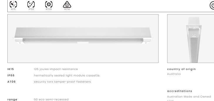
SVR050ECO-SRE0500-FXD830100-WHT product code description Extruded aluminium mounting base with durable polyester powder coat finish and impact-resistant GRP security caps Impact-resistant UV-stabilised high-transmission polycarbonate light module diffuser Serviceable replaceable and upgradable light module cassette Internal socket drive security-torx 304 stainless steel security fasteners
