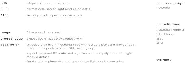
Internal socket drive security-torx 304 stainless steel security fasteners Integral energy efficient Zhaga compliant Tridonic LED modules and power supply unit Direct-fix or recessed butterfly bracket
