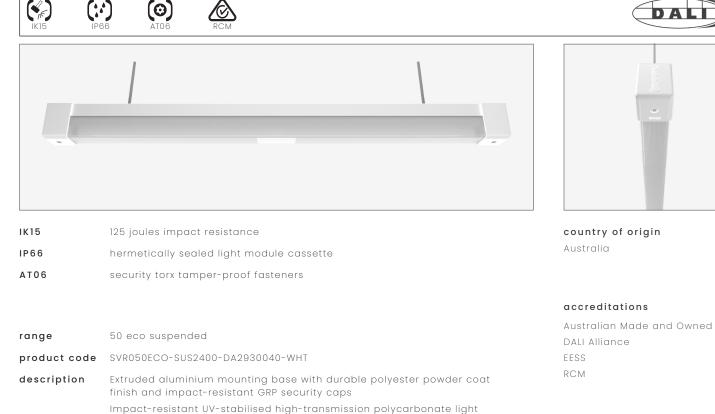
Impact-resistant UV-stabilised high-transmission polycarbonate light module diffuser Serviceable replaceable and upgradable light module cassette Internal socket drive security-torx 304 stainless steel security fasteners Integral energy efficient Zhaga compliant Tridonic LED modules and power supply unit Heavy-gauge stainless steel wire suspensions Internal stainless steel wire safety lanyards 1.0 m circular flex connection
