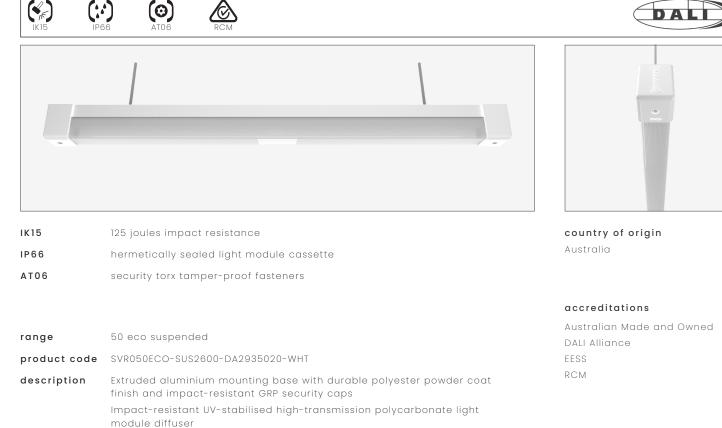
Serviceable replaceable and upgradable light module cassette Internal socket drive security-torx 304 stainless steel security fasteners Integral energy efficient Zhaga compliant Tridonic LED modules and power supply unit Heavy-gauge stainless steel wire suspensions Internal stainless steel wire safety lanyards
