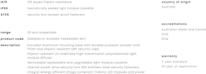
Integral energy efficient Zhaga compliant Tridonic LED mod supply unit Heavy-gauge stainless steel wire suspensions Internal stainless steel wire safety lanyards
