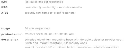
Impact-resistant UV-stabilised high-transmission polycarbonate light module diffuser Serviceable replaceable and upgradable light module cassette Internal socket drive security-torx 304 stainless steel security fasteners Integral energy efficient Zhaga compliant Tridonic LED modules and power supply unit Heavy-gauge stainless steel wire suspensions Internal stainless steel wire safety lanyards
