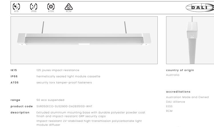
warranty 7-year standard Internal socket drive security-torx 304 stainless steel security fasteners 10-year on application Integral energy efficient Zhaga compliant Tridonic LED modules and power
