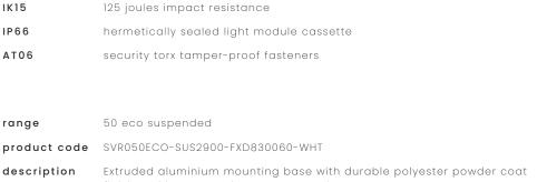
finish and impact-resistant GRP security caps Impact-resistant UV-stabilised high-transmission polycarbonate light module diffuser Serviceable replaceable and upgradable light module cassette Internal socket drive security-torx 304 stainless steel security fasteners Integral energy efficient Zhaga compliant Tridonic LED modules and power supply unit Heavy-gauge stainless steel wire suspensions Internal stainless steel wire safety lanyards 1.0 m circular flex connection
