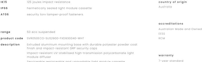
Serviceable replaceable and upgradable light module cassette Internal socket drive security-torx 304 stainless steel security fasteners Integral energy efficient Zhaga compliant Tridonic LED modules and power supply unit Heavy-gauge stainless steel wire suspensions Internal stainless steel wire safety lanyards
