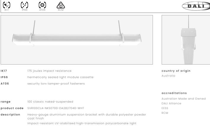
Impact-resistant UV-stabilised high-transmission polycarbonate light module diffuser Serviceable replaceable and upgradable light module cassette Internal socket drive security-torx 304 stainless steel security fasteners Integral energy efficient Zhaga compliant Tridonic LED modules and power supply unit Heavy-gauge stainless steel wire suspensions
