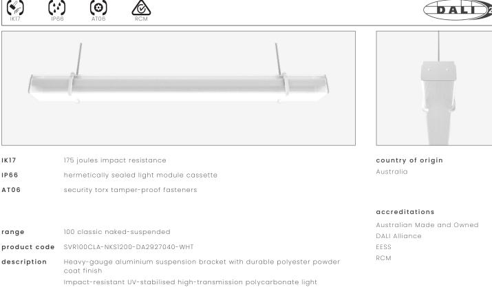
module diffuser Serviceable replaceable and upgradable light module cassette Internal socket drive security-torx 304 stainless steel security fasteners Integral energy efficient Zhaga compliant Tridonic LED modules and power supply unit Heavy-gauge stainless steel wire suspensions
