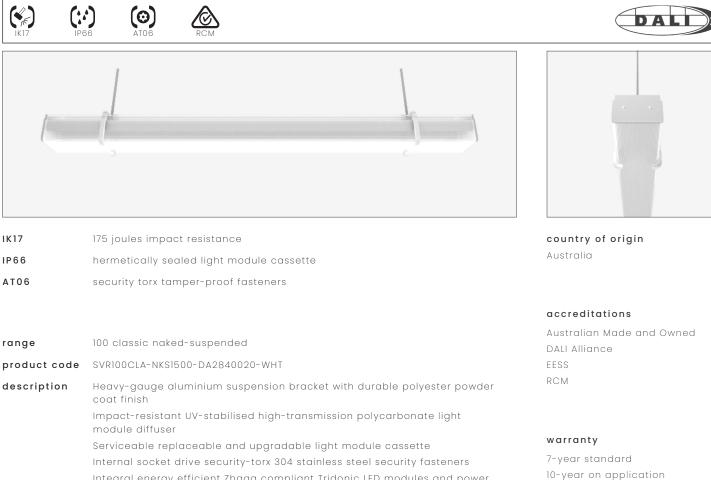
Integral energy efficient Zhaga compliant Tridonic LED modules and power supply unit Heavy-gauge stainless steel wire suspensions
