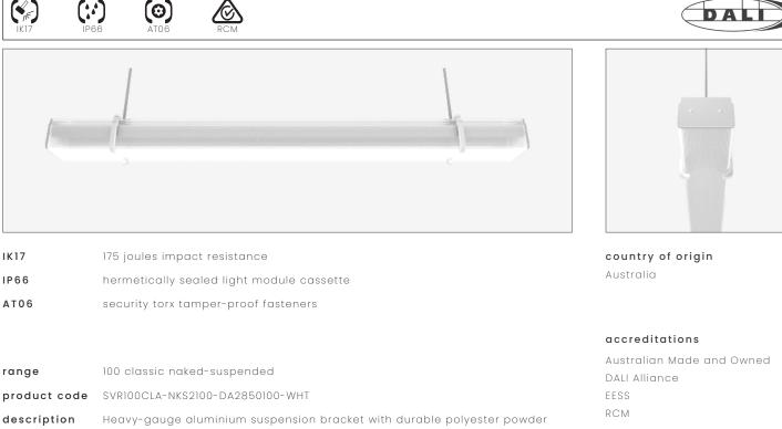
coat finish Impact-resistant UV-stabilised high-transmission polycarbonate light module diffuser Serviceable replaceable and upgradable light module cassette Internal socket drive security-torx 304 stainless steel security fasteners Integral energy efficient Zhaga compliant Tridonic LED modules and power supply unit Heavy-gauge stainless steel wire suspensions 1.0 m circular flex connection
