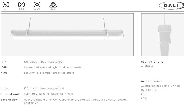
Impact-resistant UV-stabilised high-transmission polycarbonate light module diffuser Serviceable replaceable and upgradable light module cassette Internal socket drive security-torx 304 stainless steel security fasteners
