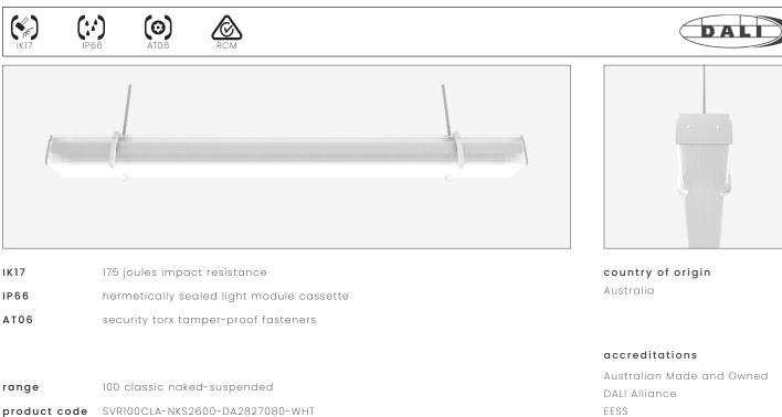
description Heavy-gauge aluminium suspension bracket with durable polyester powder coat finish Impact-resistant UV-stabilised high-transmission polycarbonate light module diffuser Serviceable replaceable and upgradable light module cassette Internal socket drive security-torx 304 stainless steel security fasteners Integral energy efficient Zhaga compliant Tridonic LED modules and power supply unit Heavy-gauge stainless steel wire suspensions 1.0 m circular flex connection
