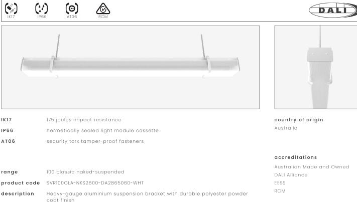
Impact-resistant UV-stabilised high-transmission polycarbonate light module diffuser Serviceable replaceable and upgradable light module cassette Internal socket drive security-torx 304 stainless steel security fasteners Integral energy efficient Zhaga compliant Tridonic LED modules and power supply unit Heavy-gauge stainless steel wire suspensions 1.0 m circular flex connection
