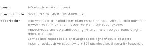
Integral energy efficient Zhaga compliant Tridonic LED modules and power supply unit Direct-fix or recessed butterfly bracket Internal stainless steel wire safety lanyards
