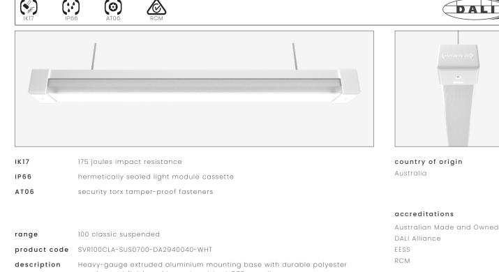
iption Heavy-gauge extruded aluminium mounting base with durable polyester powder coat finish and impact-resistant GRP security caps
